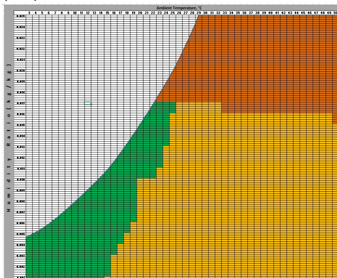
Figure 14. Operating modes of the CO 2 system enhanced with the DPC.
